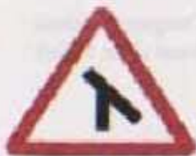
Road joins with road from the right
