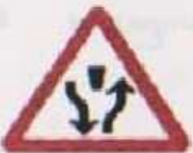
Divided Road Begins
